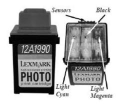
Important: Make certain that the sensors on the back of the cartridge do not get damaged.
