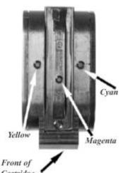
3. Insert the needle into the filling hole of the color you are refilling, (see diagram above) and push all the way towards the center of the cartridge.
