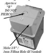
3. Some cartridges have a "filling hole" on the top sealed by a plastic or stainless steel ball bearing, as shown in photo to the right. This must be removed by pushing it into the cartridge using a pointed object such as a ballpoint pen.
