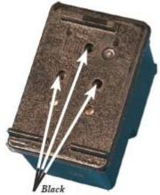
Push the needle all the way into the cartridge of the proper filling hole.
