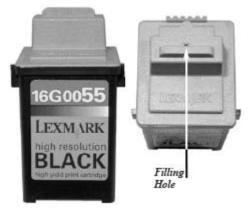
Fill the syringe with ink, insert the filling needle into the filling hole and push as far down into the cartridge. Inject approximately 20 ml of ink slowly or until the reservoir is full. After refilling and running the test pages restore the settings to economy to minimize the ink usage.
