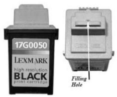
3. Fill the syringe with ink, insert the filling needle into the filling hole and push as far down into the cartridge. Inject approximately 20 ml of ink slowly or until the reservoir is full. After refilling and running the test pages restore the settings to economy to minimize the ink usage.
