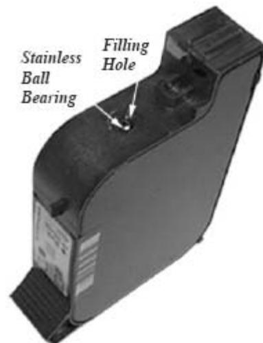
5. Replace the cartridge and run 1 - 3 cleaning cycles as per printer instructions.
