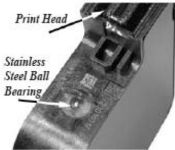
Allow cartridge to stan with the print head down for 2 minutes to draw out any excess ink and equalize the pressure in the cartridge.
