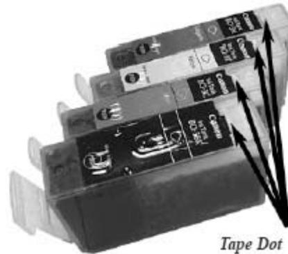
3. Use a pointed object to cut the label covering the plastic ball bearing which seals the filling hole (as shown). Use a pointed object such as a philips screwdriver or a ball point pen and push the plastic ball bearing into the cartridge.
