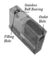
Additional Note: In some cases the sponge is deteriorated and it cannot hold the ink which will cause ink to leak out the outlet hole. If this happens an alternate method of refilling is to drip ink on to the sponge until it is soaked. (Your total page output will be less than a complete fill.)
