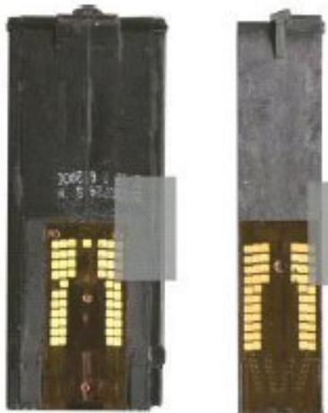
2. Place a piece of tape so that it just covers the top 4 contacts on the top left side of the contact area as shown.
